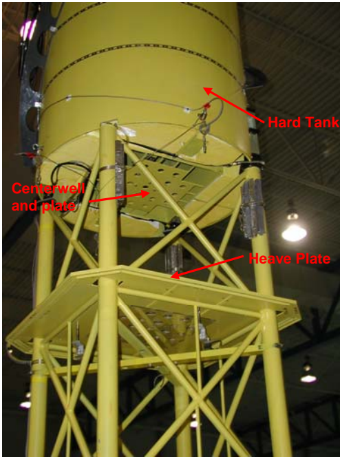
Figure 1. Spar platform. Note centerwell opening, centerwell plate and upper heave plate.
